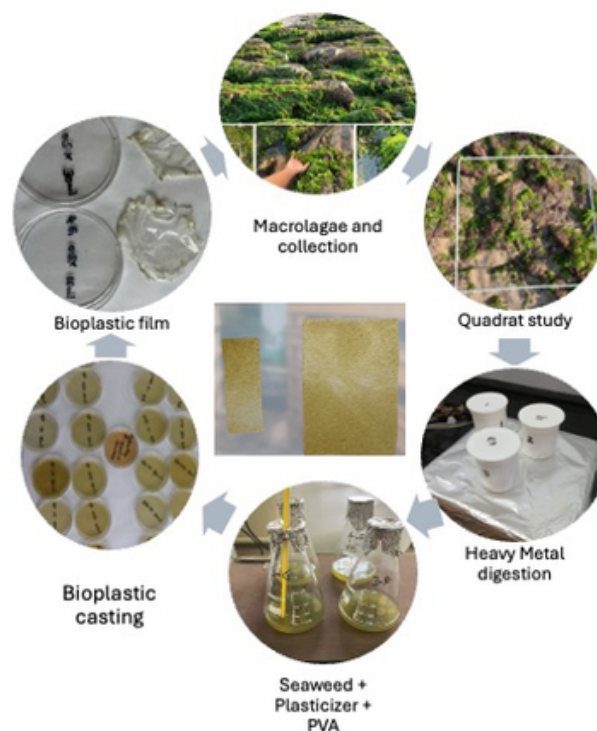
Macroalgae abundance, collection, heavy metal digestion, and preparation of bioplastic using seaweeds.
