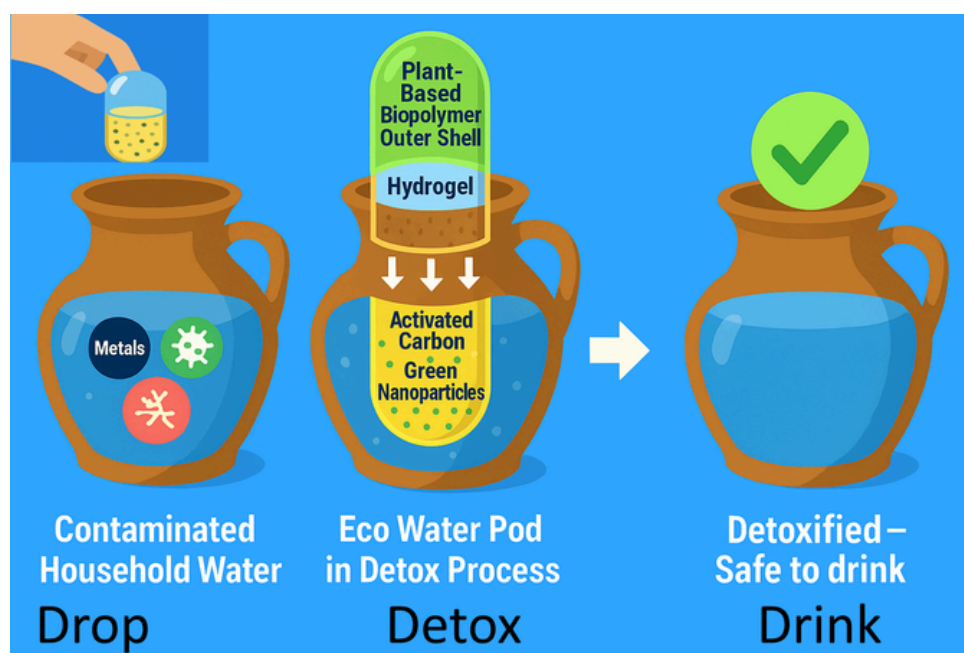
A simple “Drop–Detox–Drink” process showing how Eco Water Pods made of plant-based biopolymer hydrogels remove metals and microbes from contaminated water, making it safe to drink.
